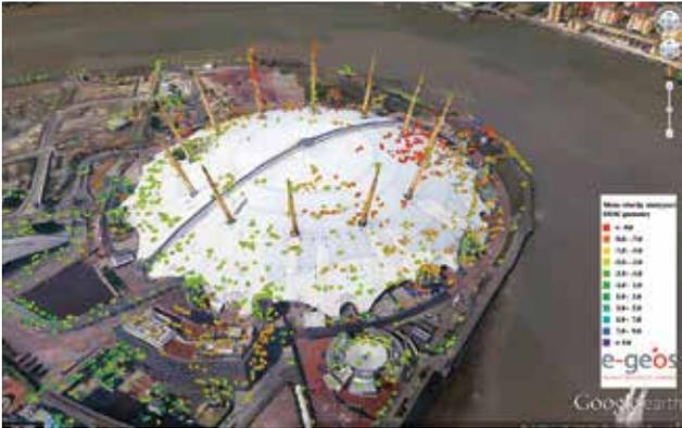
Figure 2: detecting movement at what was the Millennium Dome. (Image courtesy Telespazio, processed by e-GEOS)
