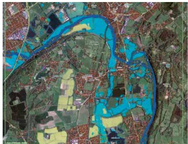
Figure 3: flood water extents extracted from radar imagery [processed by e-GEOS]
